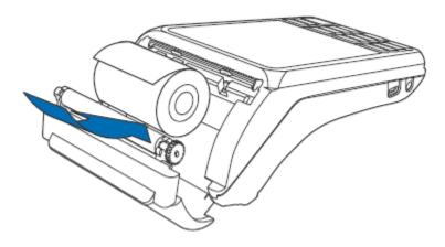
3. Pull a length of paper up over the serrated cutter and close the compartment door.
