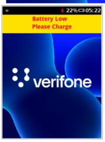
Low Battery notification, when the battery level will be less than 25%.
