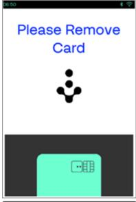
The transaction is completed, and the card can be removed. After the card is removed the status screen is displayed, until the next command is sent.
