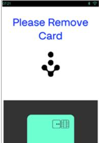
The transaction is completed, and the card can be removed. After the card is removed the status screen is displayed, until the next command is sent.
