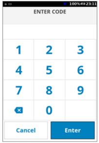
REGISTER command sends a 4-digit code to the device. Enter this code to register the POS. Once registered, the POS should run the Test MAC command to confirm the pairing worked.
