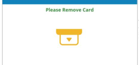
The transaction is completed, and the card can be removed. After the card is removed the status screen is displayed, until the next command is sent.
