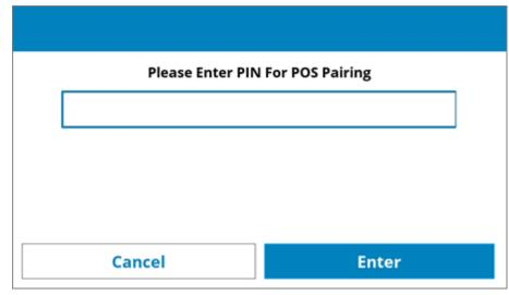
REGISTER command sends a 4-digit code to the device. Enter this code to register the POS. Once registered, the POS should run the Test MAC command to confirm the pairing worked.
