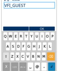
Add the network name in SSID field and press OK or Enter.
