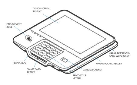
Front Panel The front panel offers the following features:
