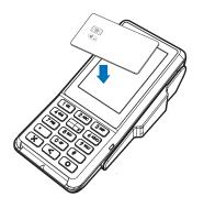
The P400/P400 Plus/P400 Dual MSR supports contactless transactions through an integrated contactless module. The terminal only becomes active for contactless smart card transactions when initialized by an application.
