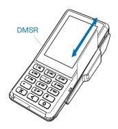
The P400/P400 Plus has a magnetic card reader that uses a triple track stripe reader and P400 Dual MSR has dual magnetic card readers that uses a dual track stripe reader. This gives the unit greater reliability over a wide range of swipe speeds and operating environments.
