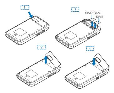
5 Inserted SIM/SAM door-remover should not be pushed behind, to release the cover refer step 3 in Figure 4.
