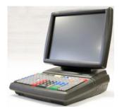
The Verifone<sup>®</sup> Topaz<sup>™</sup> XL workstation is a high-performance, reliable, point-of-sale terminal that supports peripherals such as scanners, cash drawers, PIN pads, and customer displays. The Verifone Topaz utilizes the Verifone Commander to connect to payment networks, fuel dispensers, car wash controllers, and loyalty providers. The Topaz has the ability to accept all payment options, including cash, checks, credit and debit cards, coupons, and various prepaid cards.
