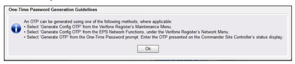
The OTP is 4 digits in length. When generated using any of the 3 methods above, it will appear on the 7- Segment status display of the site controller (displaying 2 numbers at a time; the period indicates the first set of numbers). If generated from the POS/register, it will also display on the POS screen.
