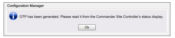
7. Read the OTP digits from the Commander. Enter the four OTP digits into the text box and then press **[OK]**.
