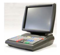
The Verifone® Topaz<sup>™</sup> XL workstation is a high-performance, reliable, point-of-sale terminal that supports peripherals such as scanners, cash drawers, PINpads, and customer displays. The Topaz utilizes the Commander Site Controller to connect to payment networks, fuel dispensers, car wash controllers, and loyalty providers. The Topaz has the ability to accept all payment options, including cash, checks, credit and debit cards, coupons, and various prepaid cards.
