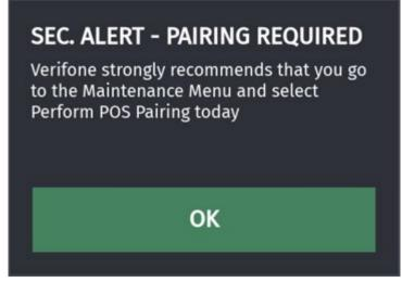
1. On the POS Workstation, navigate to CSR Func > Maintenance Menu. Press [Perform POS Pairing].
