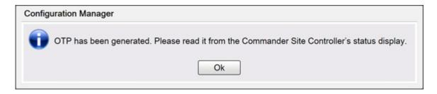
7. Read the OTP digits from the Verifone Commander. Enter the four OTP digits into the text box and then press [OK].
