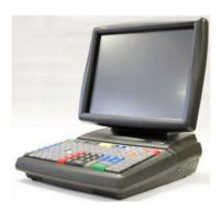
The Verifone® Topaz™ XL workstation is a high-performance, reliable, point-of-sale terminal that supports peripherals such as scanners, cash drawers, PIN pads, and customer displays. The Verifone Topaz utilizes the Verifone Commander to connect to payment networks, fuel dispensers, car wash controllers, and loyalty providers. The Topaz has the ability to accept all payment options, including cash, checks, credit and debit cards, coupons, and various prepaid cards.
