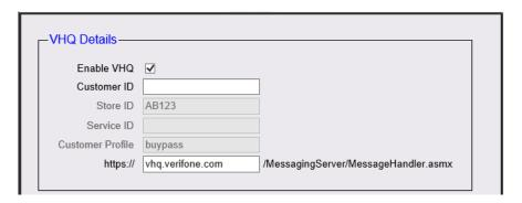
On save, the form validates customer ID and VHQ address. VHQ address can be a URL or an IP address. Customer ID can be Alphanumerical characters up to 64 characters. If validation is not successful, an error message is displayed.
