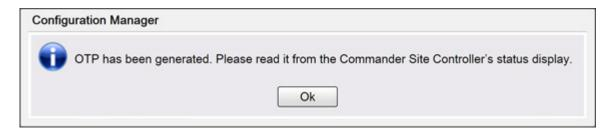
4. Read the OTP digits from the Verifone Commander, Enter the four OTP digits into the text box and then press [OK].
