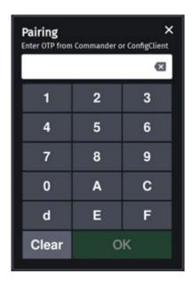
12. Navigate to Configuration Client > Security > Site Security. Press [Retrieve Pairing OTP].
