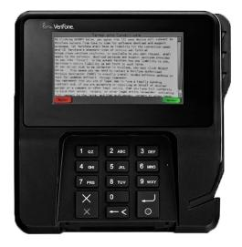
Should a customer reject the agreement after updating the ViperPAY version and want the Service and Maintenance feature later, they can enter into System Mode on the PIN pad, navigate to "Enable VHQ default" and change the value to 1. They will then need to run the application from the PIN pad home screen and accept the Terms & Conditions prompt. This must be completed for each PIN pad.
