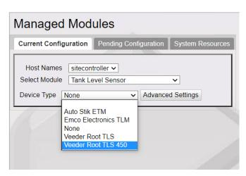
Veeder Root TLS 450 is the more advanced version of Veeder Root TLS, which can support 16 tanks and has more alerts incorporated.
