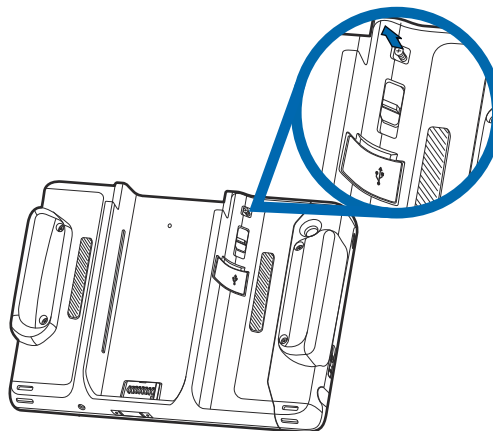
Figure 13 Loosening Screw to Unlock Release Button
