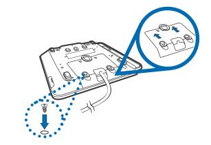
Figure 5 Closing Cable Compartment with Cable Cover
