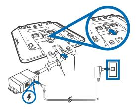
Figure 4 **Multiport Cable Connected on the Rear of the Unit**
