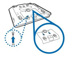
Figure 3 **Removing Cable Cover**
