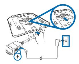
Figure 8 Connecting Base Cable to Device
