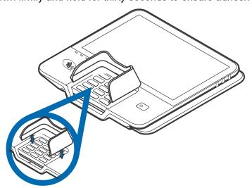
Figure 13 Installing the Privacy Shield
