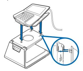
Figure 18 Docking Terminal onto the Stand
