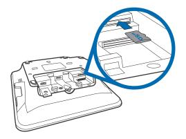
Figure 7 Inserting a Micro SD Card
