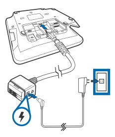
Figure 9 Connecting Base Cable to the Terminal
