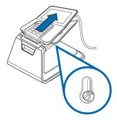
Figure 20 Undocking Terminal from the Stand
