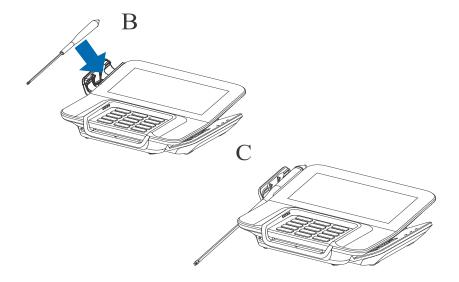
Figure 16 Placing the Stylus Holder
