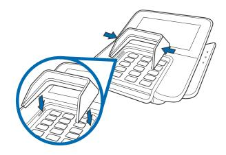
Figure 14 Installing the Privacy Shield
