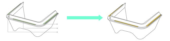
Step 3: Peel to remove all the three liners.
