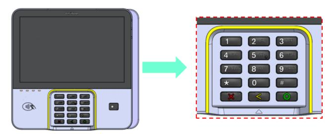
Step 2: Clean the yellow surface using an alcohol cleansing pad.
