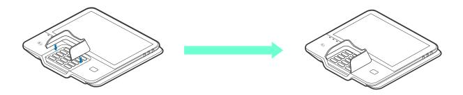
Step 4: Align the privacy shield with the device to ensure it is straight along the top. Once aligned, exert downward pressure on the top edge of the privacy shield for ten seconds. After you have secured the top, exert downward pressure on the left and right sides.
