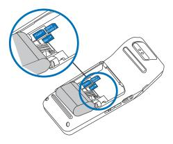
4 Turn the battery back into the compartment and place it in the slot as shown in Figure 5.
