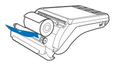
3 Pull a length of paper up over the serrated cutter and close the compartment door.
